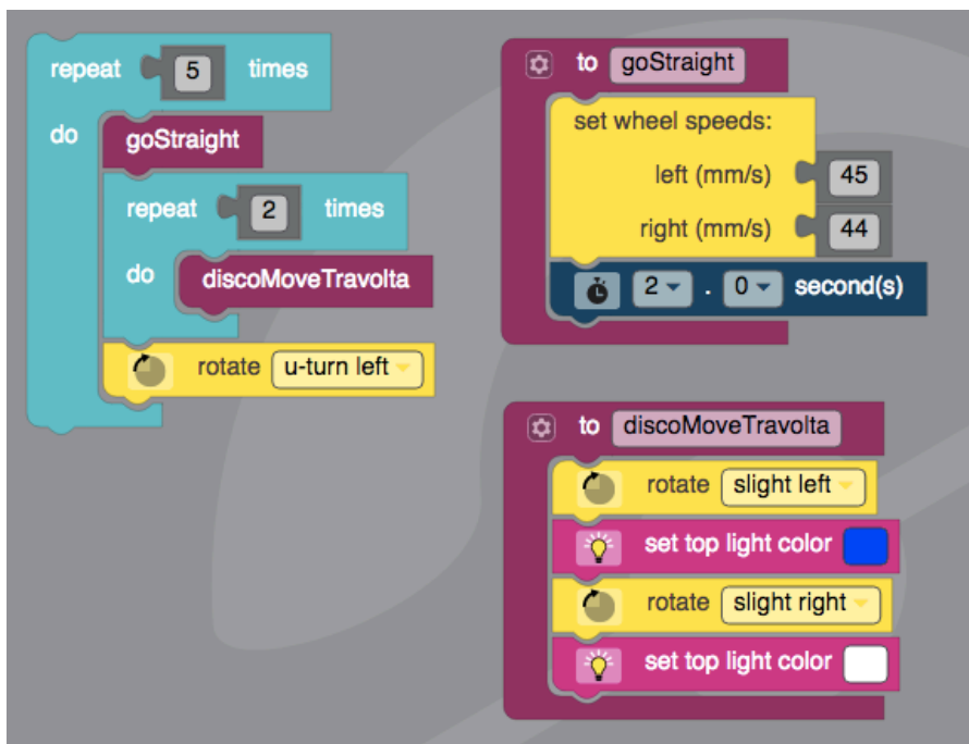
Example: Ozobot does Travolta's Point Move dance from Saturday Night Fever top left: the code block that's actually running; top right, bottom right: functions that only run when you "call" the code "discoMoveTravolta" and "goStraight"
