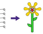
Last, attach the battery holder to the flower. Make sure the red wire inserts into the red part of the flower and the black wire is inserted into the yellow outside ring. Turn on the battery holder to light up the flower.
