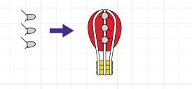
5 Last, insert the red wire into the right half of the balloon and the black wire into the left. Turn on the battery holder to light up the balloon!
