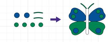
Next, attach the long legs of LEDs into the left side of the butterfly's wings, with the smaller legs going into the right side.
