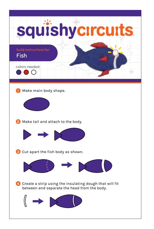
5 Next, make the fins and attach them to the body as shown. 6 Insert an LED for the eye. Be sure to place the longer LED leg into the dough with the red battery holder inserted. 7 Turn the battery holder switch on to light up the LED. for additional ideas, recipes and more, go to: squishycircuits.com
